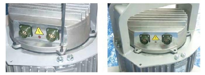
Lean Pc Board to connect power line and probe – ATTENTION to colours: U - BLACK / V - GREY / W - BROWNAssembly PC board to motor and clamp it.
