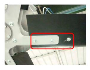
SCREW M8x60 TCEI NUT 8,4x24 h2 SELFBLOCKING BOLT M8
