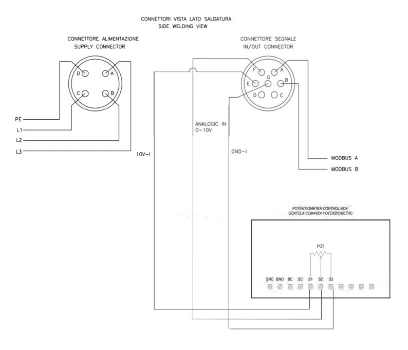
NB: It is necessary pull the A and B wires down to the control box for the Modbus connection, used for maintenance and diagnostic actions.
