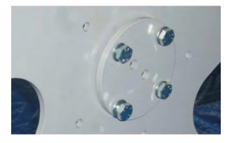
INSERT PLATE INTO BLADE SUPPORT USING SCREWS M10x45 TE NUT. 10,5x20 h2
