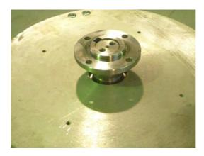
AFTER DISASSEMBLED BLADE SUPPORT, DISASSEMBLY
