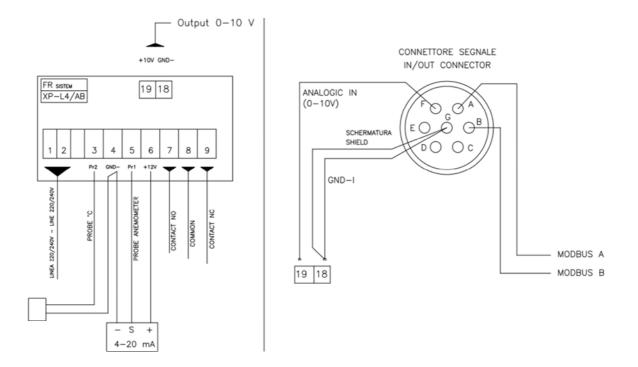
**NB:** It is necessary pull the A and B wires down to the control box for the Modbus connection, used for maintenance and diagnostic actions.
