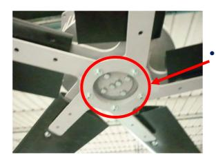
Fix without tightening the 5 central screws of the reinforced spider to the main one, with bolts and nuts
