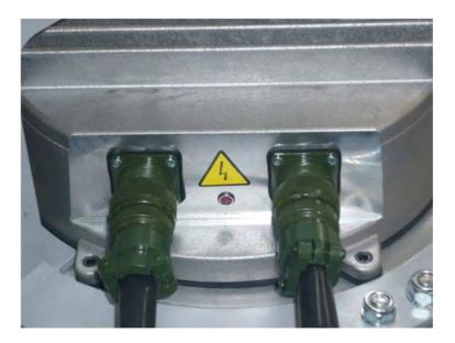
DISCONNECT POWER DISCONNECT BOTH OF TWO CONNECTORS FROM FAN Diassembly Fan – POWER – Operation with motoinverter connectet to the roof
